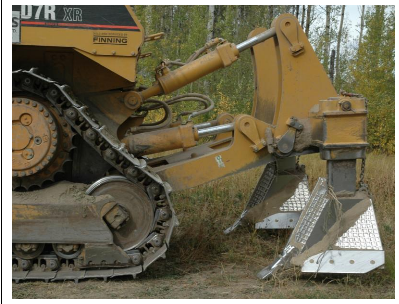
Figure 4. Pair of prototype RipPlows on a Caterpillar® D7R used to till forest roads and wellsites in Alberta. Soil can be tilled to depths up to 0.90 m and produce a gain in soil elevation of 0.15 m.
